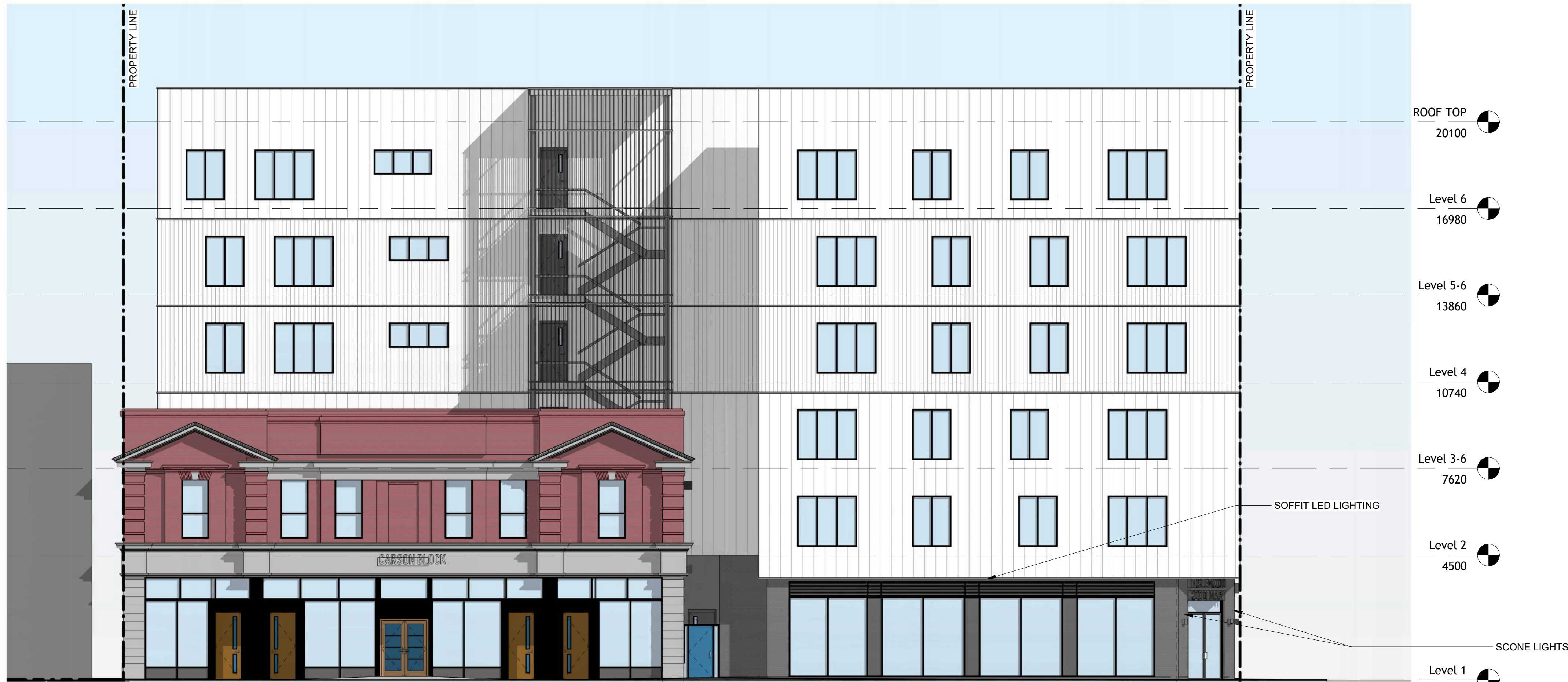
1 SOUTH ELEVATION - COLOUR DP3.03 1 : 100
